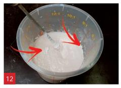
Stir the mixer till all lumps have disappeared (± 1 min.) resulting in a smooth material.
