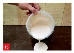
A1 is ready for laminating, casting or spraying. Processing time ± 20 minutes.
