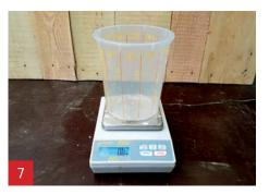
Place a cup on the scale. Calibrate the scale together with the cup (0.0 g).
