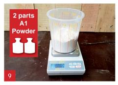
Weigh 2 parts of A1 Powder. In this example we use 1000 g A1 Powder.
