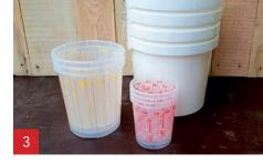
Set up (plastic) cups for mixing the materials (A1 Liquid, A1 Powder).
