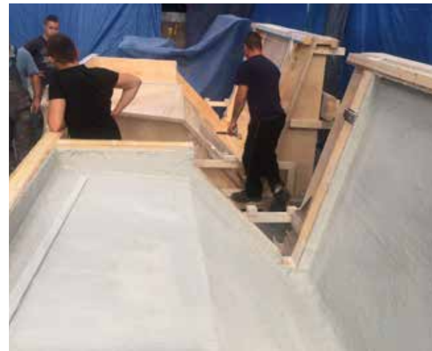
A1 element laminated in the mould
