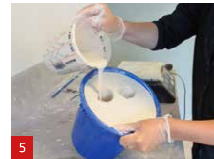
5 Slowly pour some of the A1 along the edge into the opening(s). Let the A1 flow through the shape in all directions to reduce air entrapment. Turn and tap on the bucket so the A1 fills the empty spaces properly and any air bubbles arise. Pour in the remaining A1. Again, tap on the bucket and fill to where necessary.
