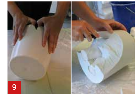
9 The A1 is dry, but not yet fully cured. Therefore, carefully remove the alginate where the pouring holes are located.
