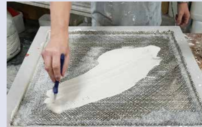
To laminate, you have to work wet in wet. A quick way to apply A1 is with a brush or roller.
