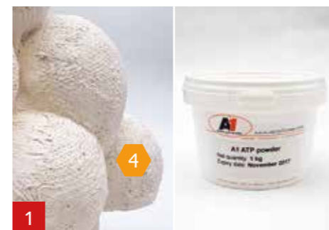
1 Creating a smooth finish on the object. First weigh 1 part A1 Liquid and 2 parts A1 Powder and mix until all lumps have disappeared. Set up the ATP powder.
