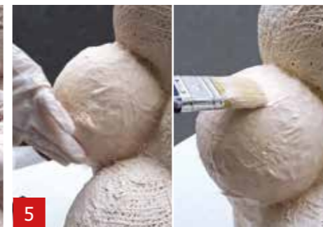
5 The C-veil must be covered with a layer of A1 by hand or brush.
