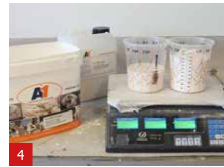
4 Weigh 1 part A1 Liquid and 2 parts A1 Powder and mix. The A1 is ready as soon as you run out of lumps or air bubbles. Tip: Gently tap the bucket on a hard surface to release air.
