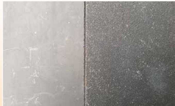
A1 panel with sand directly after demoulding.
