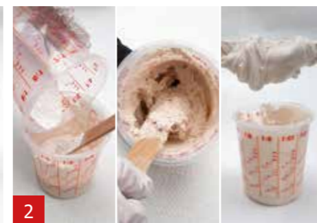
2 Add as much ATP powder as needed into the A1. Stir firmly till all lumps have disappeared. The A1 texture can be made as a paste or as a putty.
