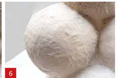
6 For a more smooth finish you can add a second layer of C-veil.
