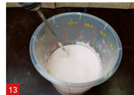
13 A1 is ready for use when all lumps have disappeared.
