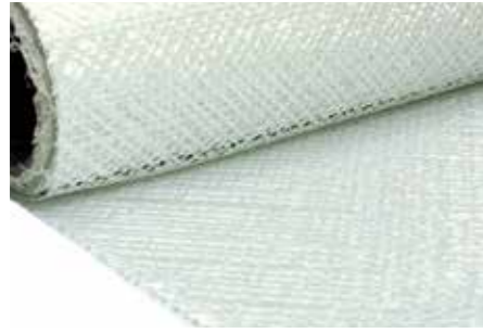
A1 Triaxial glass fibre 160 gr/m 2
