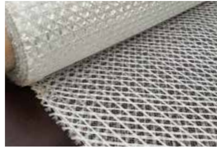
A1 Quadriaxial glass fibre 210 gr/m 2
