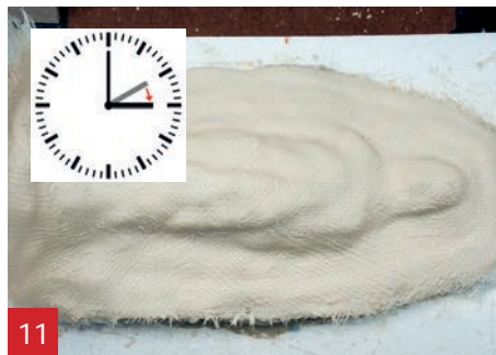
Let the A1 support mould dry for 60 minutes.
